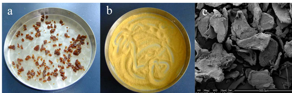
Figure 3. The images of dried chitosan products (CH-3, drying temperature = 60 °C). (a) optical image of product from direct drying; (b) optical image of product from drying with freeze-thaw pretreatment; (c) SEM image of product from drying with freeze-thaw pretreatment. [Color figure can be viewed in the online issue, which is available at wileyonlinelibrary.com .]
